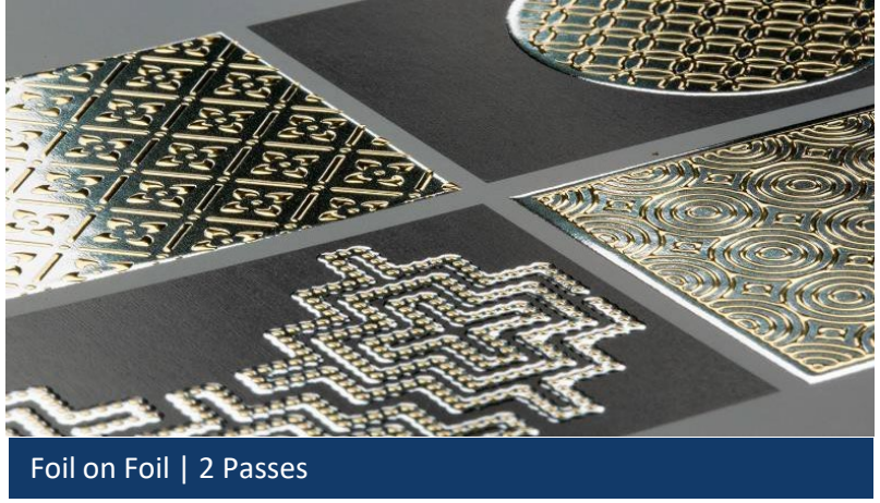
Textured substrate causes imperfections in the foil. The busy design helps hide the imperfections.
